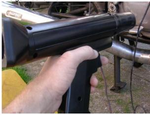
And it must be attached to one of the four ignition cables.
