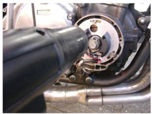
The mark should match the first 2-3 mark. If not, move the base plate.
