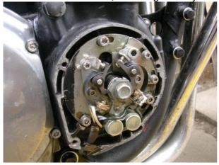
First remove the retainer bolt for the automatic ignition advancer. In the centre you see a smaller hex – which is the bolt, and a larger hex, which is used to turn the motor.
