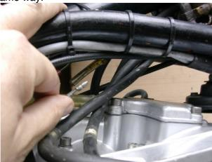
Connect the white and black wires in the same way the old wires were connected, and connect the red wire to a 12V switched with the ignition key. The orange wire to one of the ignition coils could be used.
