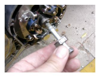
Remove the base plate, by removing the 3 screws holding it:
