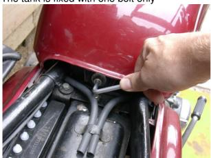
Remember to disconnect the fuel line and the vacuum hose before removing the tank.
