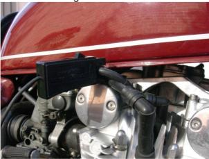
Here it is attached to cylinder 3, and I will use the 2-3 checkmark. Had I used cylinder 4, I would have used the 1-4 checkmark.
