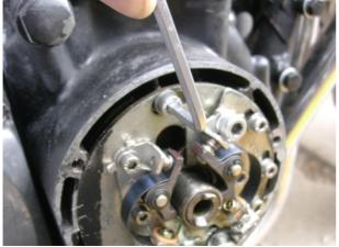
Remove the base plate, and take out the advancer:
