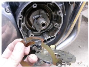
Behind the base plate, is a gauge with marks for ignition positions. This will be reused.
