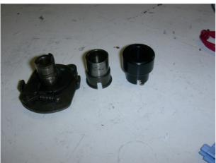
The new rotor is shown to the right, and the old eccentric guide in the middle.
